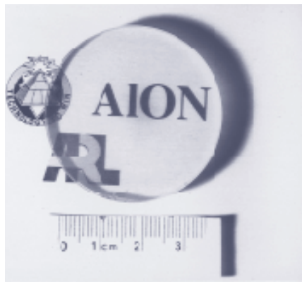
Figure 3: A hot pressed four-inch diameter, 0.44" thick spinel plate and 1.63" diameter, 0.25" thick AION produced at ARL
