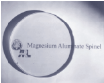
Figure 3: A hot pressed four-inch diameter, 0.44" thick spinel plate and 1.63" diameter, 0.25" thick AION produced at ARL
