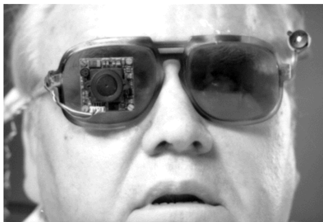
Figure 1. Blind volunteer with sub-miniature TV camera mounted on the right lens of his sunglasses, and the laser-pointer (position monitor) on the left temple piece.
